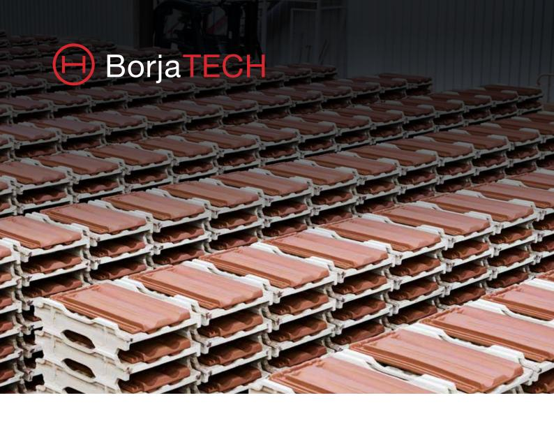
The manufacturing process of Tejas Borja, with plaster molds and H cassettes, confers to our products a very perfect and detailed definition with greater clay compaction, a very low absorption and extremely strong.
